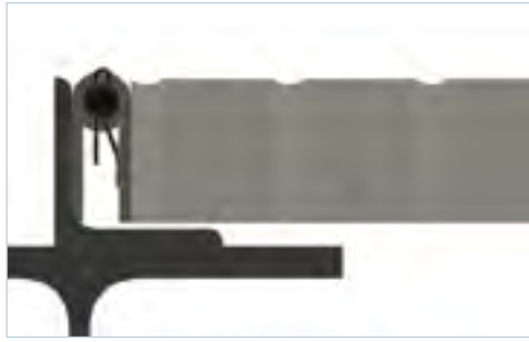
Hinge B 1680 Composed of: • 2 hinge plates • 1 hinge pin • 2 U-washers • 2 cotter pins
